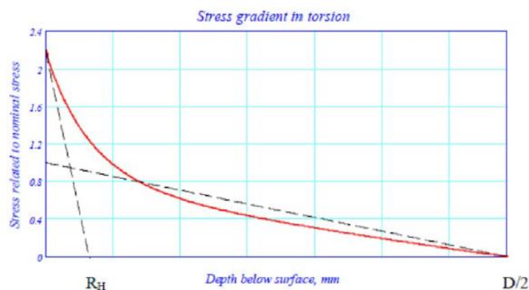
Figure 2.3.23: Torsional SCF in the crankpin fillet as a function of depth. The corresponding SCF for the journal fillet can be found by replacing R_H with R_G and D with D_G
